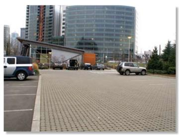
it to be re-absorbed into the ground for natural cleaning and filtering before reaching the lake. The Discovery Center features two such measures: a pair of bioswales flanking the building and a parking lot surfaced with Mutual Materials<sup>®</sup> Eco-Stone<sup>®</sup> permeable pavers.
